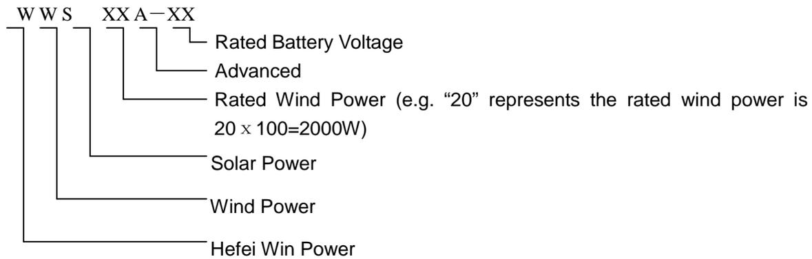
eg. WWS 10A-48-E (1000W Advanced Wind/Solar Hybrid Controller, Battery Voltage is 48V)
